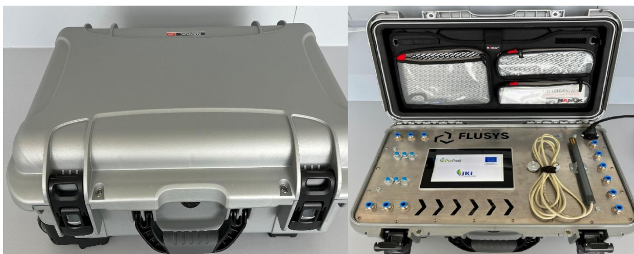
Figure 2: Portable 6-channel headspace collecting device (HSCD) for collecting VOCs.
