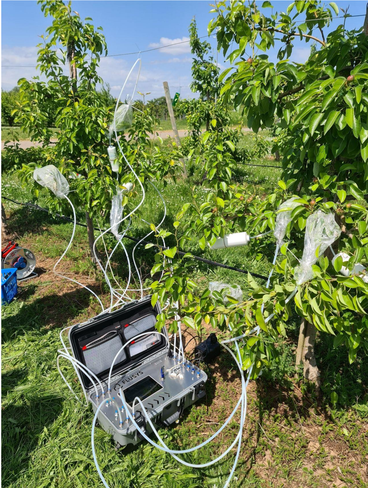
Figure 4: Portable 6-channel headspace sampling device for collecting VOCs of pear trees in the OLS (right side) and CLS (left side) modes.
