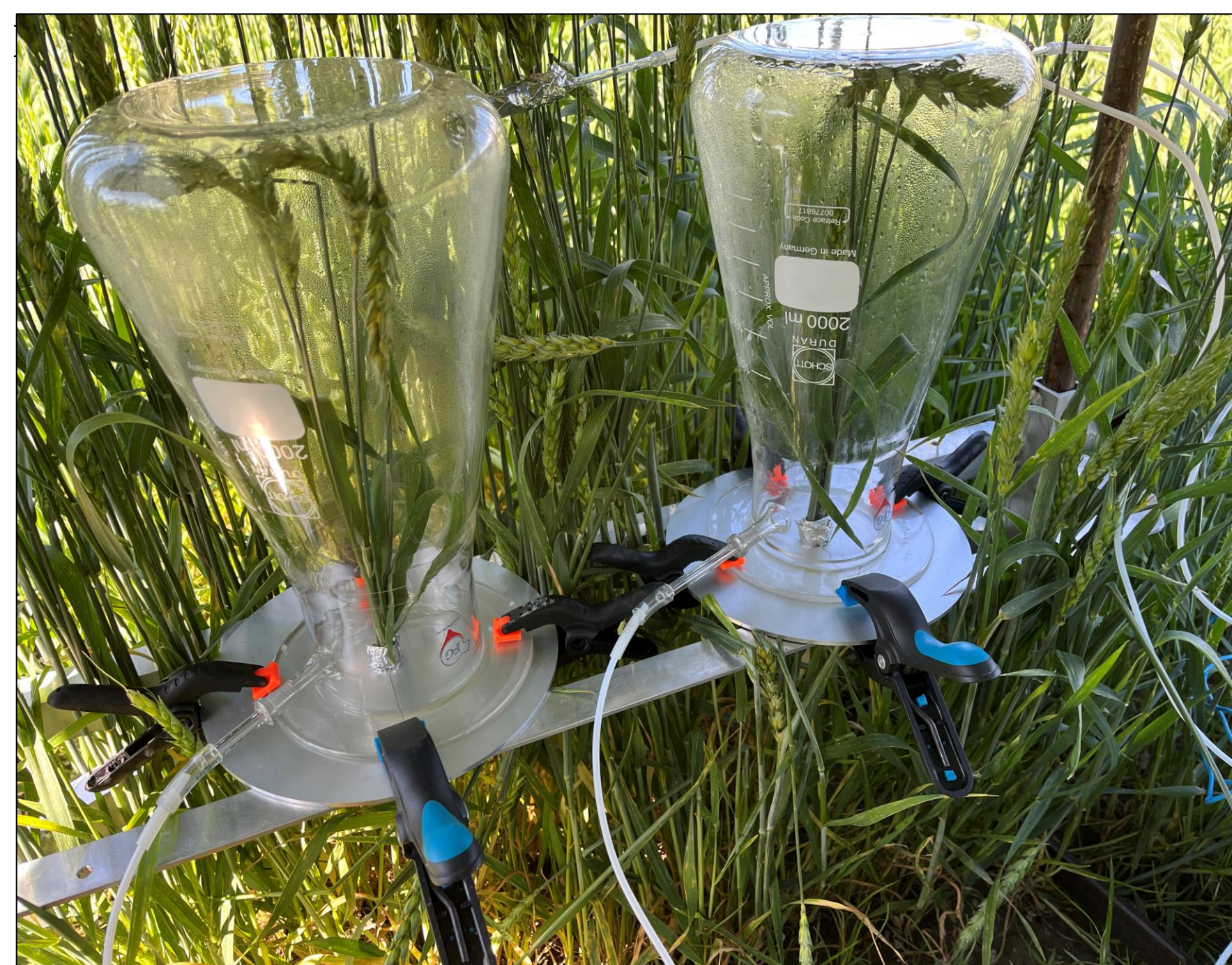
Figure 1. VOC collection in the field: Charcoal filtered air flows over two groups of 4-5 wheat plants and is collected on SuperQ filters for 24 hr.
