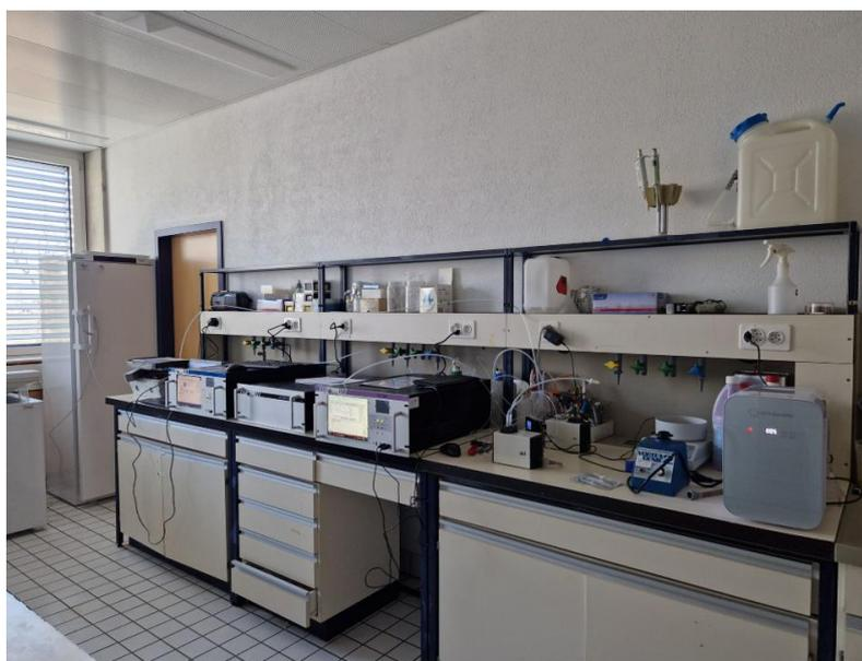
Figure 3-22: Analytical systems used at UNINE for characterization of Fall Armyworm-Induced Volatiles in Maize
